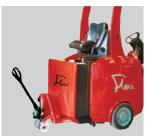
Low rear lift off or roll off for fast changeovers. Good access for battery topping. No electric motors, brakes or pumps underneath.
