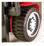
Flexi AC 1200 front twin drive wheels provide excellent grip and traction in slippery conditions when fully loaded. Continental MC20 super-elastic finger tread tyres for extended service life and resistant to damage.
